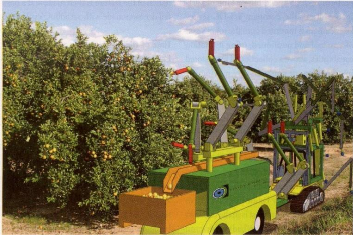
FIGURE 3. To automate the process of orange picking, Vision Robotics has proposed the development of a stereo camera-based system that will use multiple cameras placed at the end of multi-axis arms to create a virtual 3-D image of the entire orange tree.
